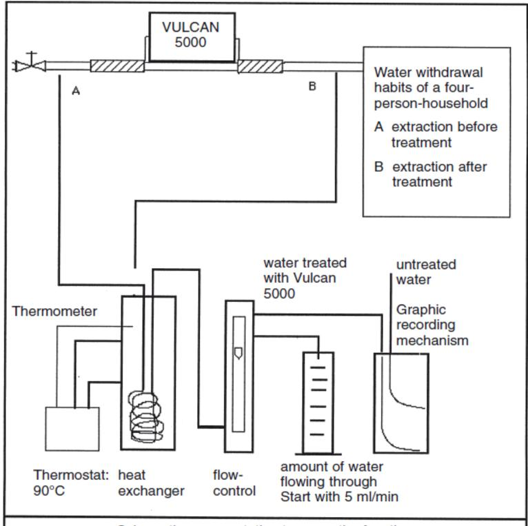
Schematic representation to prove the function of the water-treatment device VULCAN 5000 (Only one of the two tests is mentioned in the schematic representation)
